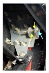
Adjust the nuts (yellow arrow) closer together. Tighten the draw bolt (blue arrow) moving the rotor cage to the right (as if sitting in drivers seat). Tighten draw bolt until the rotor bars ting the concaves when you spin the rotor, then back off until the ting stops. Tighten the bolts on the front and rear module carrier supports 103 ft lbs
